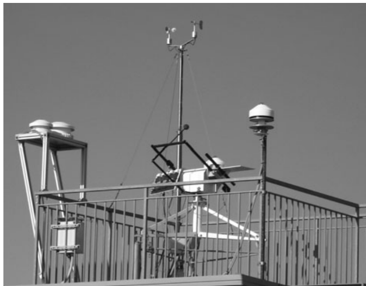
Figure 1. View of the solar-weather unit of the ESTER station; on the left are the two spectroradiometers.
