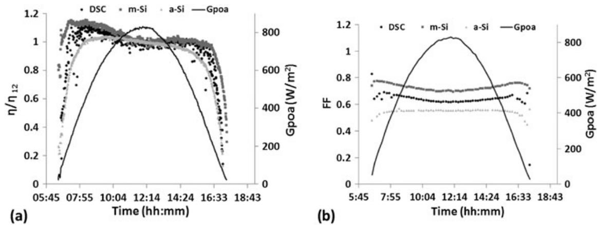
**Figure 8.** Performance of dye sensitized solar cells, multi-crystalline silicon, and amorphous silicon modules for a sunny day in October 2011: (a) relative efficiency and (b) fill factor.
