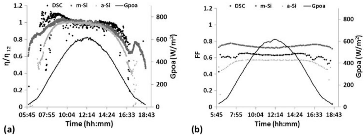
**Figure 7.** Performance of dye sensitized solar cells, multi-crystalline silicon, and amorphous silicon devices for a sunny day in August 2011: (a) relative efficiency and (b) fill factor.
