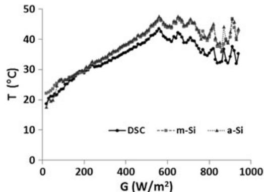
**Figure 5.** Average back of the module temperatures evaluated at different plane of array irradiance classes.
