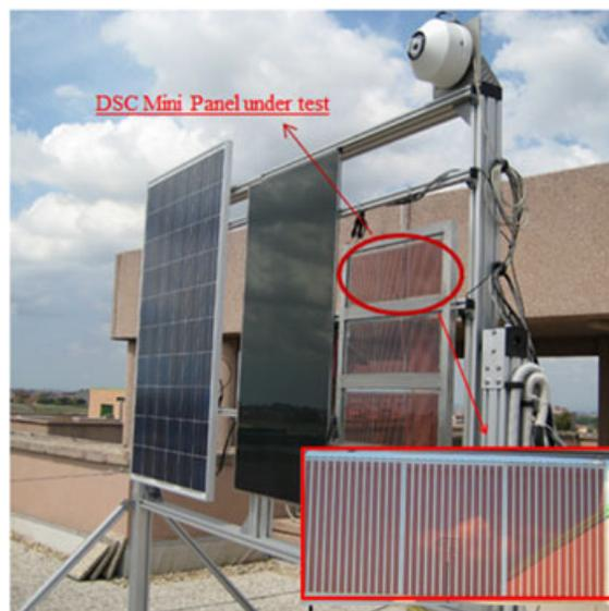
**Figure 1.** View of the photovoltaic modules arranged on the dedicated frame and the detail of the dye sensitized solar cells (DSC) mini-panel.
