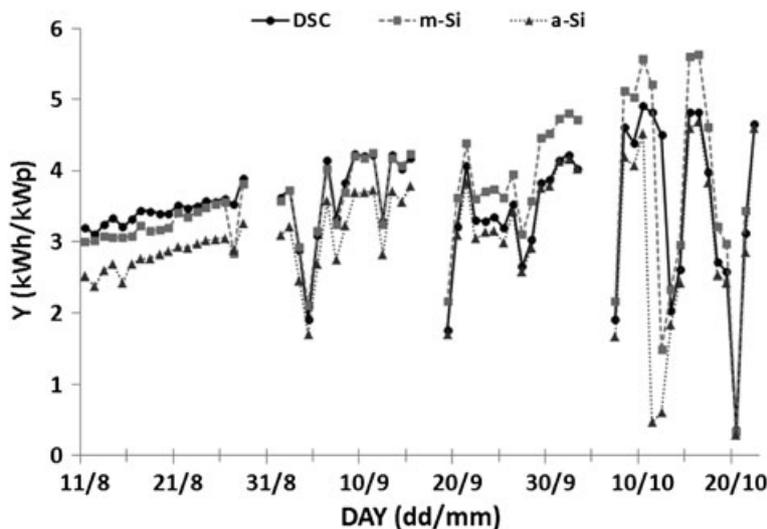
Figure 9. Daily yield calculated for dye sensitized solar cells, multi-crystalline silicon, and amorphous silicon modules.
