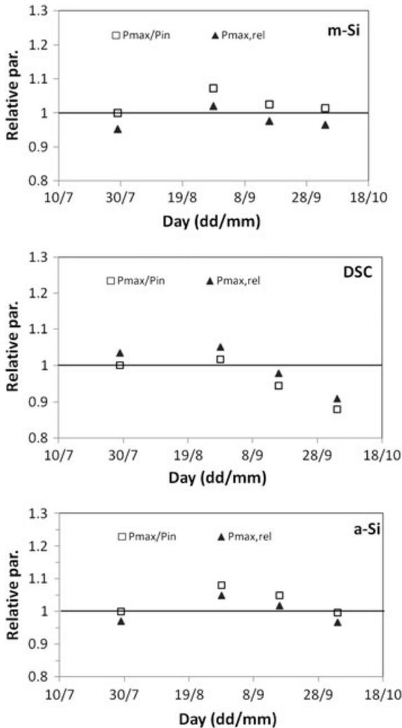
**Figure 6.** Variation of  $P_{max}$  translated at standard test conditions (STC), normalized by the nominal (manufacturer) maximum power ( $P_{max,rel}$ ) and for the measured  $P_{max}$  at STC obtained at the beginning of the campaign ( $P_{in}$ ) versus time for the three devices during the period of test. DSC, dye sensitized solar cells.
