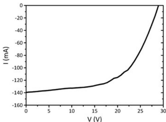
**Figure 2.** *I*-*V* curves of the dye sensitized solar cells mini-panel after the lamination procedure.
