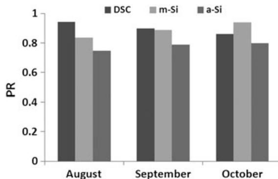
**Figure 12.** Monthly performance ratio ( $PR$ ) calculated for dye sensitized solar cells, multi-crystalline silicon, and amorphous silicon modules for the period of test.
