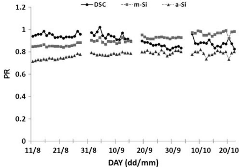
Figure 11. Daily performance ratio (*PR*) calculated for dye sensitized solar cells, multi-crystalline silicon, and amorphous silicon modules for the period of test.
