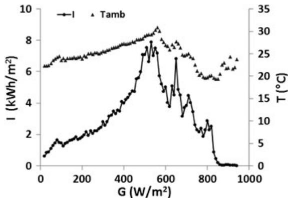
**Figure 4.** Irradiation ( $I$ ) and average ambient temperature ( $T_{amb}$ ) measured at different plane of array irradiance classes.
