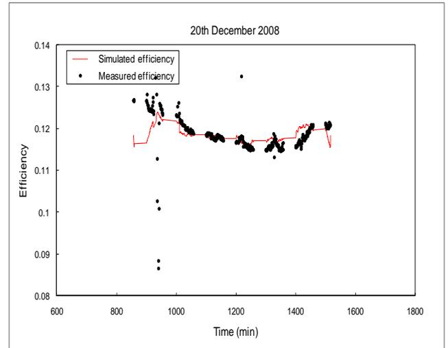
**Fig. 10:** Comparison of simulated and measured efficiencies, tilt 65° facing South, 20<sup>th</sup> December 2008.
