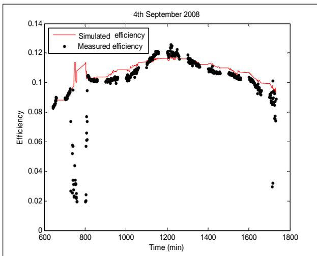
**Fig. 9:** Comparison of simulated and measured efficiencies, tilt 20° facing South, 4<sup>th</sup> September 2008.
