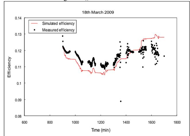
**Fig. 11:** Comparison of simulated and measured efficiencies, tilt 40° facing South, 18<sup>th</sup> March 2009.
