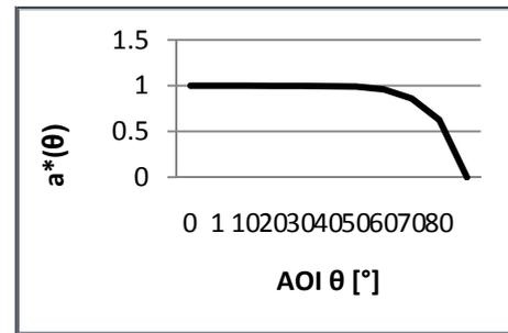
Fig. 5: Absorption rate of the glass cover of a PV module vs angle of incidence.
