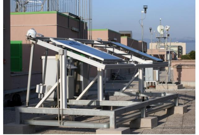
**Fig. 7.** View of the FTA Laboratories facility ESTER used for experimental validation of the simulation model.
