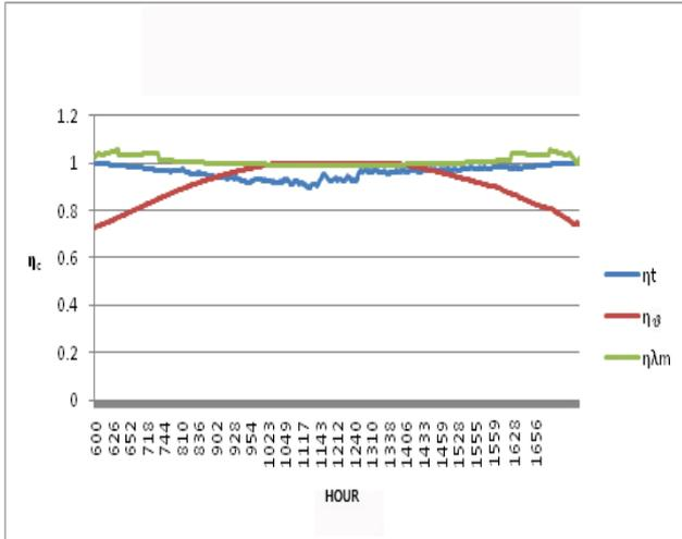
**Fig.12:** Single effects of the corrective coefficients on the nominal efficiency, 29<sup>th</sup> June 2008.
