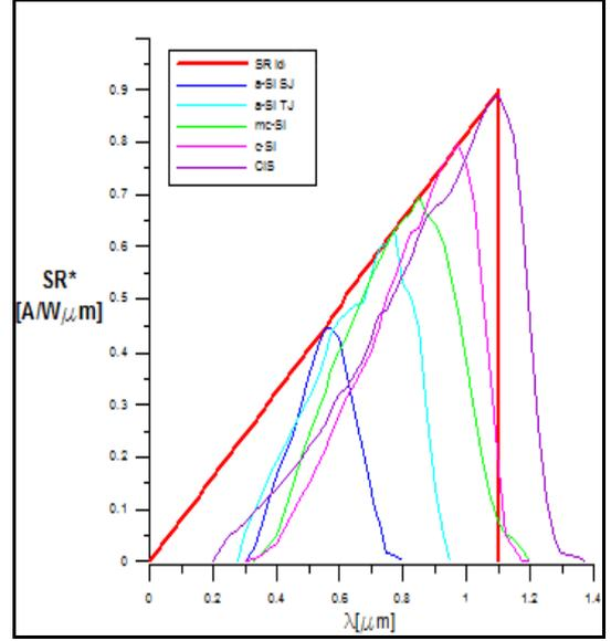
Fig. 4: Spectral response of various cells.
