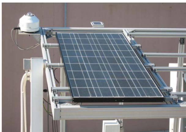
**Fig. 1.** View of the reference PV panel used for experimental validation of the simulation model.
