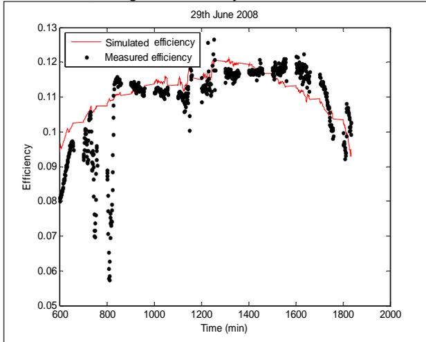
**Fig. 8:** Comparison of simulated and measured efficiencies, tilt 20° facing South, 29<sup>th</sup> June 2008.
