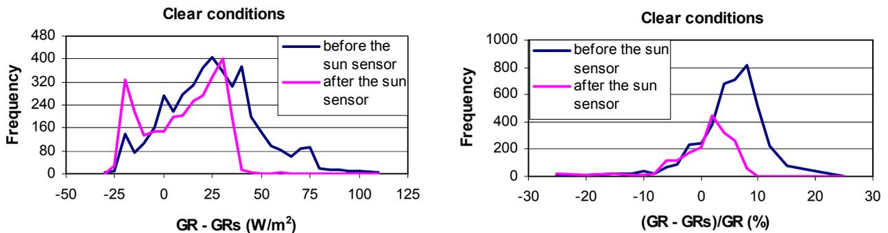
Fig. 8. Histograms of data collected for clear conditions before and after the sun sensor installation.
