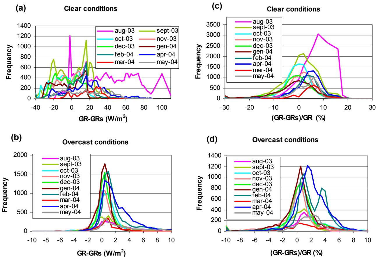
Fig. 6. a) and b) absolute  $GR-GR_s$  difference histograms for clear and overcast conditions, respectively; c) and d) relative  $GR-GR_s$  difference histograms for clear and overcast conditions, respectively.
