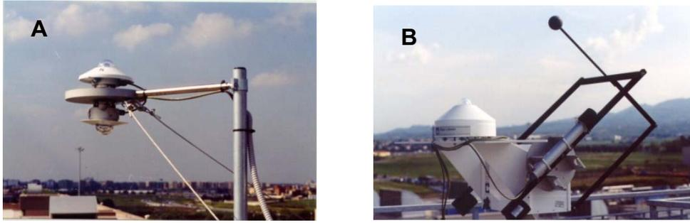
Fig. 2. Solar radiation instruments: A) albedometer; B) pyranometer for diffuse radiation measurements and pyr heliometer mounted on the 2AP suntracker.
