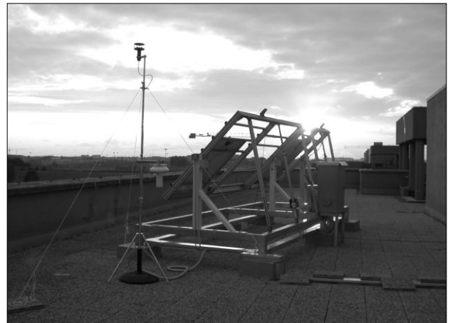
Figure 1. The ESTeR Stand for the Outdoor Testing of Solar PV Panels.
