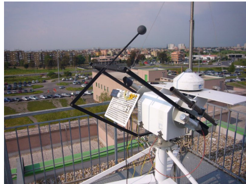
Fig. 1. Sun tracker with the cell support plate at ESTER facility.
