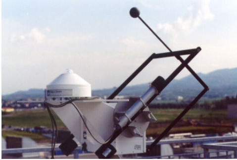
Fig. 2. Sun tracker with pyrheliometer and shaded pyranometer at the solar station.
