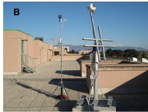
Fig. 3. a) Fixed stand mounted on the roof top of the Engineering building; two PV polycrystalline silicon modules are presently monitored; b) sun tracker for PV modules (with no modules mounted) and in-plane pyranometer.
