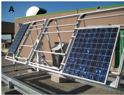
Fig. 3. a) Fixed stand mounted on the roof top of the Engineering building; two PV polycrystalline silicon modules are presently monitored; b) sun tracker for PV modules (with no modules mounted) and in-plane pyranometer.
